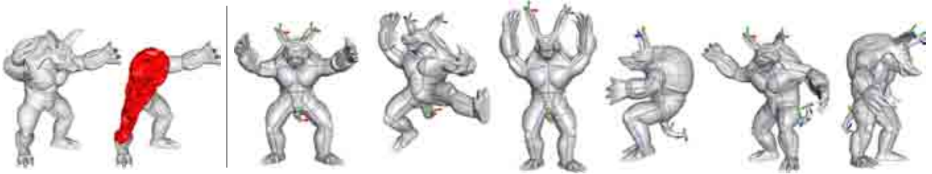
Figure 13: This example uses a human skeleton embedded in the Armadillo. The skeleton does not control the tail or the ears, but points are easily added to control them for additional expressiveness in each pose. Left: a cutaway of the Armadillo shows the graded tet mesh produced by TetGen. The inner tetrahedra are much larger than the surface ones, which keeps the discretization complexity reasonable.
