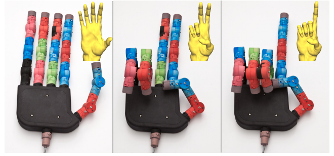
Figure 16: Our design generalizes to customized splitters like this hand. The friction control of the 14 attached joints allows the device to remain in pose as the user poses the Chimpanzee Hand.
