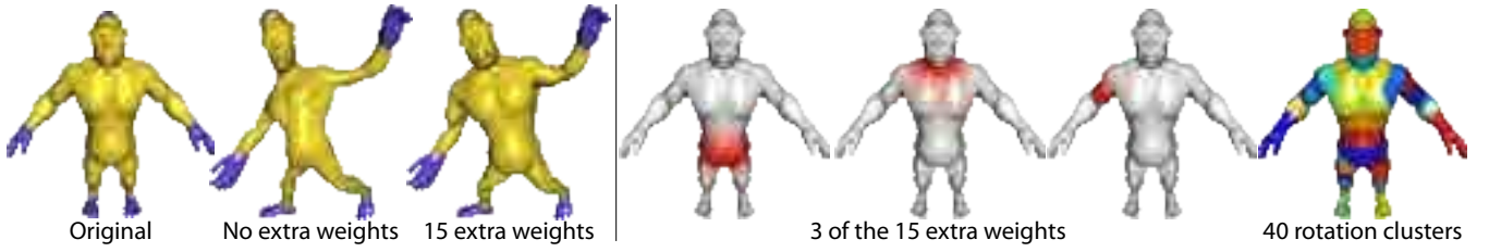
Figure 13: With five fully constrained region handles, our method reduces to LBS with its volume loss issues. Enriching our subspace with 15 additional weight functions (shown in red) allows our method to find more natural deformations.
