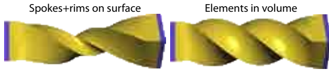
Figure 10: Our reduced model preserves the nature of different energy functions: spokes and rims (left) behave like thin shells, while tetrahedra (right) correspond to volumetric elasticity.
