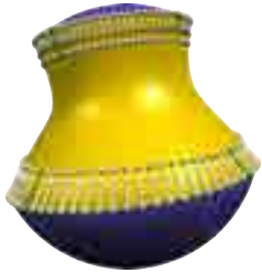
Figure 13: Blending between two spherical caps, with controllable sharp features introduced using tangent conditions.
