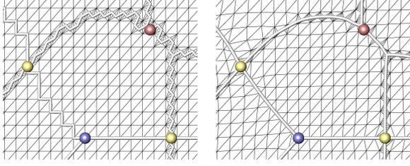
**Figure 6:** The parametric embedding of the simplified separatrices may be jaggy (left) and is smoothed by Laplacian mesh optimization (right).
