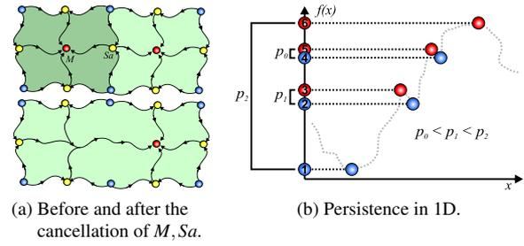
Figure 4: Persistence-based simplification by removing pairs of critical points.
