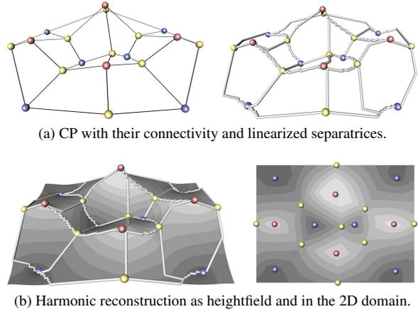
**Figure 5:** Constructing a faithful preview of the smoothed scalar field. The abstract connectivity of the simplified Morse-Smale complex (top left) is supplied with valid values by linearly interpolating between the endpoints of each separatrix (top right). A harmonic function is then computed with the separatrices as boundary conditions (bottom). Refer to Figure 9a for the input scalar field.
