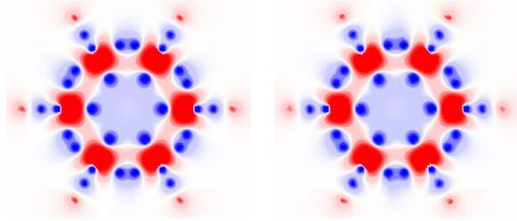
**Figure 8:** *Electrostatic field of the Benzene molecule.* The original data set (left) has been reconstructed (right) without topological simplification. The PSNR is 50.8 dB.
