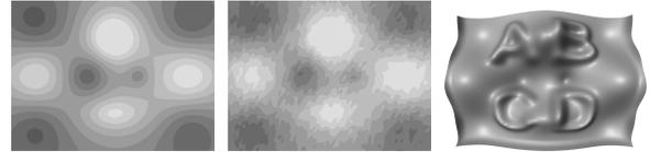
(a) The original synthetic function (left) is corrupted by additive noise (middle) and by an overlay displacement field (right, displayed as a heightfield).
