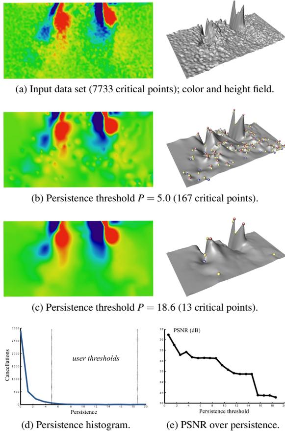
**Figure 10:** Experimentally measured data set showing the instantaneous vorticity at the outlet of a combustor (flow direction from top to bottom). The size and overall shape of the major features at the burner outlet (top) are preserved while the noise has been successfully removed.
