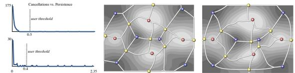
(c) Persistence histograms of the two test cases with the user-specified thresholds (left); the reconstructed results for both the noisy (middle) and the overlay (right) tests.
