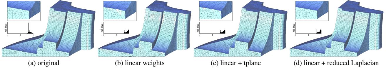
Figure 6: Triangle optimization on an input mesh (a) with distinct sharp features. Using linear weights (b) breaks the sharp features, and using (2D) tangent plane constraints (c) cannot resolve the problem, since these features would require 1D or zero dimensional (positional) constraints. Instead, we reduce the weight on Laplacian constraints of feature vertices (d).
