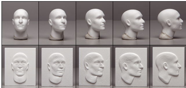
Figure 16: Multiple views of the Head model (80k vertices), rotated by 22.5 degrees and constrained to a thickness of 2 mm.
