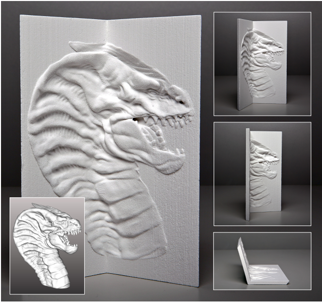
Figure 4: Appearance-mimicking surface of the Dragon Head model constrained to carve a V-shaped, thin geometry.
