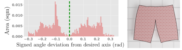
Fig. 16. A skirt pattern piece (Fig. 2, top) is split by a dart, resulting in conflicting desired grain alignment on each side. The global rotation chosen by our parameterization accommodates for both sides, despite being optimal for only a small area. On the left we show a histogram of the signed angle between the warp direction and the prescribed desired alignment.
