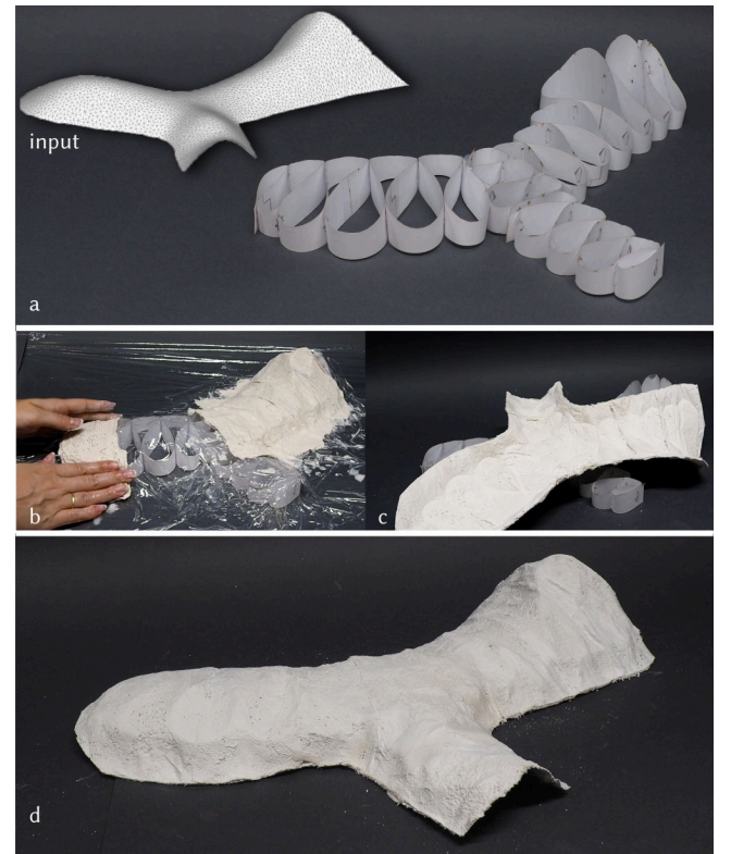
Figure 14: Our ruffles could be used as formwork for architectural shells. We show a miniature version of the (a) supporting ruffles, (b) on which we apply plaster, and (c) after removing the ruffles, we (d) obtain the original 3D shell.
