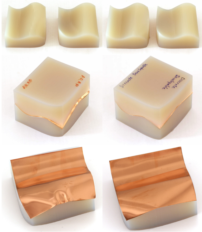
Fig. 14. Validation by fabrication. We 3D-printed a “sandwich” (top row) whose inner cut surface is the result of deforming a flat square using ARAP (left column) and our editing system for discrete developable surfaces (right column) using the same (soft) positional constraints. We cut two squares out of a thin copper sheet with the dimensions of the initial model before deformation, and we sandwiched these squares in the fabricated pieces (second row). Not surprisingly, since the ARAP result is not developable, the sheet wrinkles and buckles (bottom left), while our result exhibits pure bending (bottom right). Note that our result is smooth everywhere except at the boundary, where a cone-like kink is created in the digital model to remedy the doubly curved ARAP surface.
