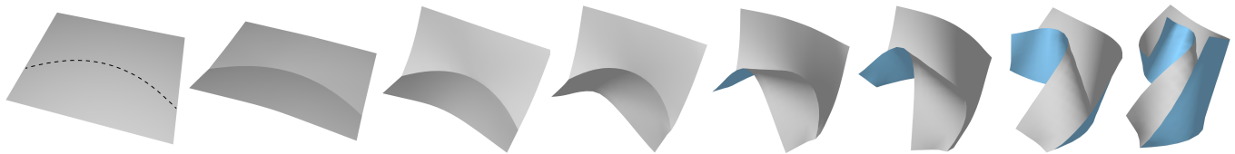
Fig. 1. We develop a theory for shape space exploration of DOG nets, which are discrete developable surfaces parameterized by orthogonal geodesics. Our study results in a characterization of this shape space and an algorithm to discretize smooth flows on DOGs, as used in the above animation. The first three frames were created using our editing system, and the rest were generated using a curve-constraining flow , deforming the surface by constraining a curve that lies on it.
