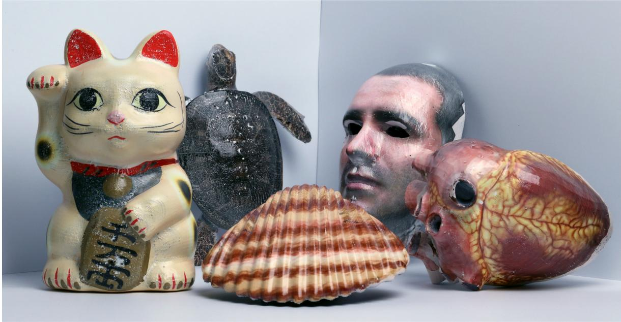
**Figure 11:** A photograph of texture mapping physical objects via hydrographics using our algorithm and mechanical setup.
