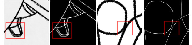
Figure 12: Input drawings (left and middle-right) present some challenging regions. Centerlines (middle-left and right) predicted by our model accurately represent them.
