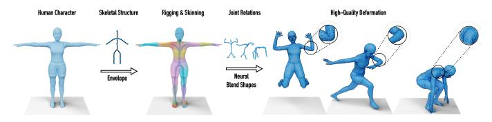
Fig. 1. Our neural skeletal articulation network learns to rig and skin an input character with arbitrary connectivity, and generates neural blend shapes. Our framework produces pose-dependent displacements that result in high quality deformations, especially in the joint regions.
