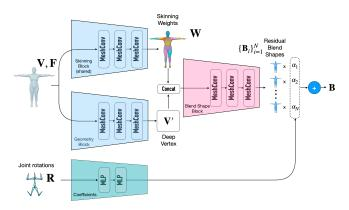
Fig. 4. The residual deformation branch predicts blend shapes and blending coefficients based on the input mesh connectivity and input joint rotations. The network learns to estimate blend shapes for arbitrary mesh connectivities and blending coefficients that are conditioned on the joint rotations.
