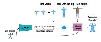
Fig. 5. Inference time. Given a new character, we can extract skin, rig, and blend shapes within a single forward pass of our network. To animate the character we need only a small network that calculates pose dependent blend shape coefficients. Conforming to standard skeletal animation models enables direct plug-and-play application in standard animation software.
