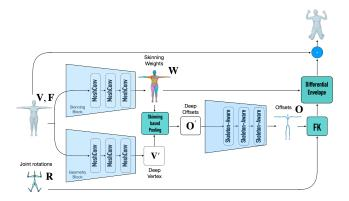
Fig. 3. The envelope deformation branch. Given a mesh in T-pose (V, F) and joint rotations (R), our network infers the skinning (W) and rigging (O) parameters via indirect supervision by observing the articulated character vertex positions.
