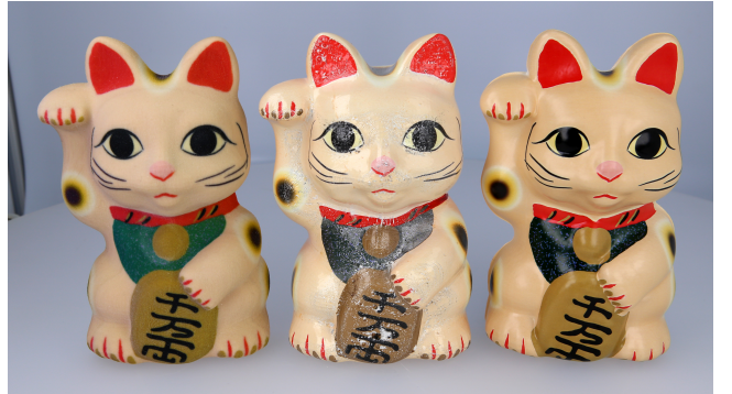
Figure 7: Our replica of the cat model (right) has a superior surface quality to that created with a ZCorp 650 powder printer [3dsystems 2016] (left) or hydrographic transfer [Panozzo et al. 2015] (middle).
