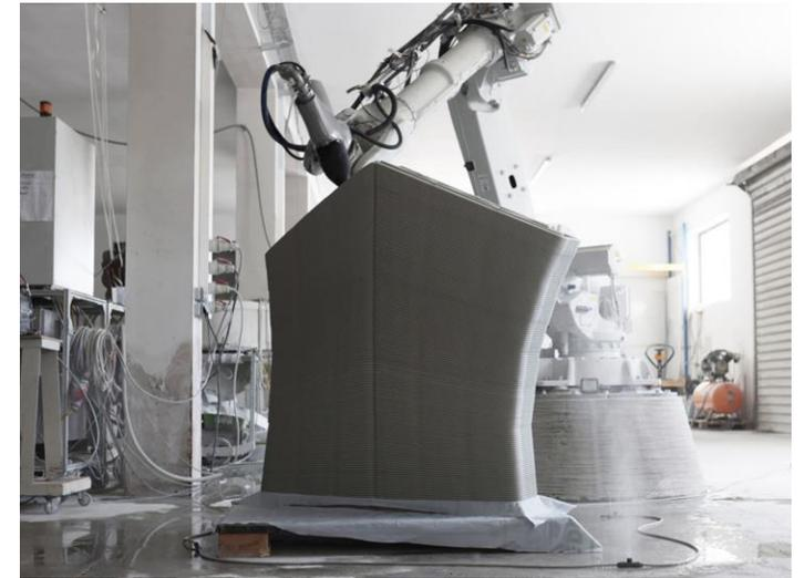
[3D printed unreinforced masonry bridge](#), BLOCK research group (ETHZ)
